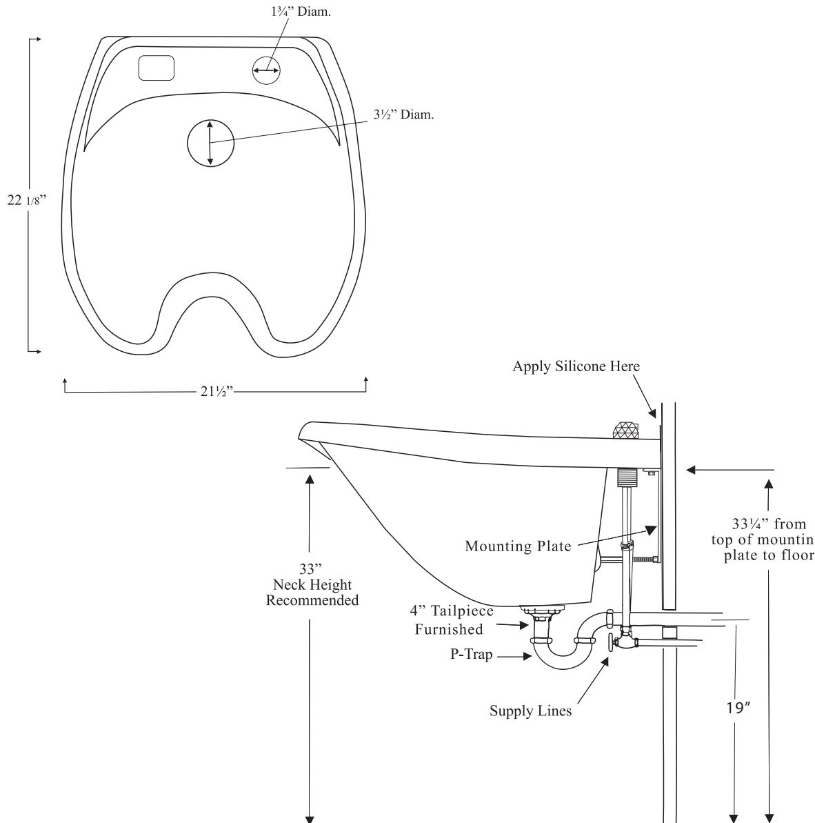
When installing in wet styling booths or cabinets refer to the manufacturer's specification sheet to determine how far the waste plumbing and water supply lines should extend from the wall to outer face of cabinet. The depth of the cabinet will determine this specification.
